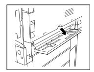
4 Adjust the paper guides to the size of the paper, and then load the paper so that the front side of the paper (the side facing up when the package was unwrapped) faces down. Lightly slide the paper into the feed slot as much as possible so that it is ready to be fed into the copier.
